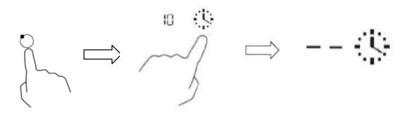
5. When the time is set, it will begin to count down immediately. The display will show the remaining time and the timer indicator will flash for 5 seconds.
