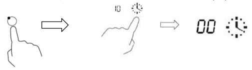
5. When the time is set, it will begin to count down immediately. The display will show the remaining time and the timer indicator flash for 5 seconds.
