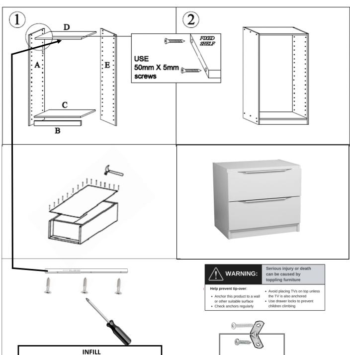
YOU WILL NEED TO RETRIEVE THE INFILL, USING 3 X 30mm SCREWS PROVIDED, ATTACH THE INFILL TO THE UNDER-SIDE OF THE CAM SHELF BEFORE PUTTING YOUR SHELF INTO PLACE.
