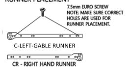
PLACE YOUR RUNNERS INTO THE DESIGNATED HOLES MAKING SURE THE WHEEL IS FACING TO THE FRONT OF THE GABLE. HOLE POSITION NO 1 & 8, .
