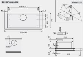
Method of Installation: Built into overhead cupboards
