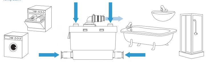
The Grey Water Pump will activate automatically following the inflow of waste water from any of the above fixtures.
