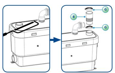
To connect to a lid inlet, cut off the sealed cap with a Stanley knife or hacksaw and connect using the rubber connector (B) provided. Tighten with the metal hose clips (G).
