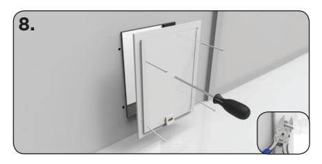
8. Screw inner door frame into door/panel. Tighten with a Phillips head screw driver. If screws protrude trim the ends to be flush. WARNING: Over tightening of screws will cause damage.
