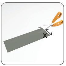
6. Measure the thickness of the door/panel and add 10mm (x) so the tunnel protrudes 5mm on each side. If required, cut partitions down to correct size.
