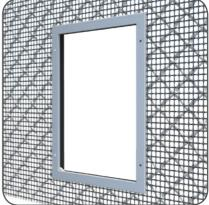
3. Fit all 4 partitions into outer door frame, use duct tape to secure the corners then place into opening.
