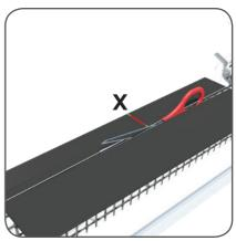
2. Measure the thickness of the door/panel and add 10mm (x) so the tunnel protrudes 5mm on each side. If required, cut partitions down to correct size.
