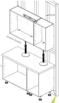
Caution: Please ensure all cabinets are screwed into your timber stud wall using a minimum of 65mm timber screws. If attaching to concrete, brick, steel or any other substrates seek advice from your hardware specialist.
