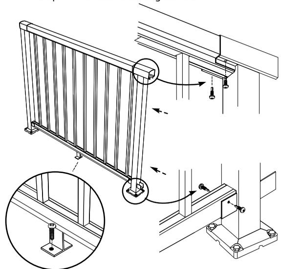
**▲IMPORTANT** To ensure that the balusters remain engaged in the rails, you must install a base rail support for each balustrade section. To install the base rail support, insert it into the bottom channel of the base rail (as shown in Step 1), slide it to the centre position and secure it to deck surface using fasteners.
