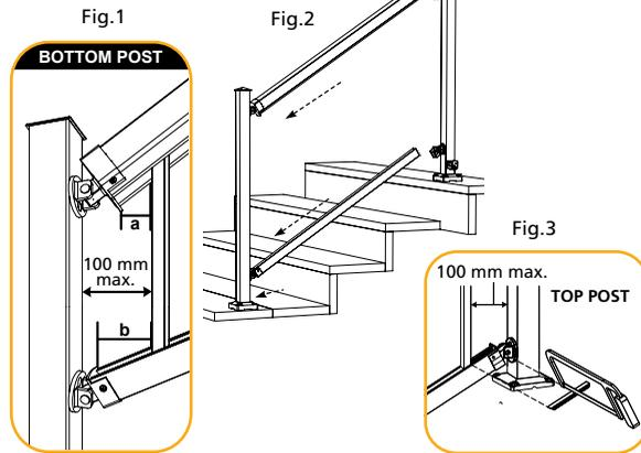
**PRO TIP:** To ensure equal spacing at each post, cut the first and last spacers in the hand and base rails to a length that ensures equal spacing between the end balusters and the posts.
