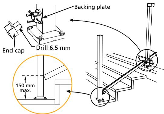
**2** Cut the handrail to the same length as the base rail and fit the UBs onto the handrail. Use two **stair balusters** to position the handrail. Mark the locations of the UBs on the posts. Remove the handrail from position and the UBs from the handrail. Drill 5.5 mm pilot holes into the posts and use the flat head screws to attach the UBs to the posts. Temporarily move the bottom post to place the hand and base rails into the UBs. Secure the UBs to the rails at the bottom post only.
