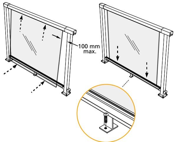
**IMPORTANT** To ensure that the glass panel remains engaged in the rails, you must install one base rail support for each balustrade section. To install the base rail support, insert it into the bottom channel of the base rail (as shown in Step 3), slide it to the centre position and secure it to deck surface using fasteners.
