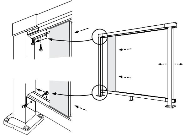
**4** Insert the rails into the second post. Position and fasten the second post in place (see table on pg. 4 & 5). Ensure that the post is plumb. Secure the rails to the second post with self-drilling screws. Repeat Steps 1-4 for each remaining section.
