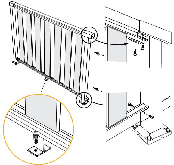
**IMPORTANT** To ensure that the glass panels remain engaged in the rails, you must install a base rail support for each balustrade section. To install the base rail support, insert it into the bottom channel of the base rail (as shown in Step 1), slide it to the centre position and secure it to deck surface using fasteners.
