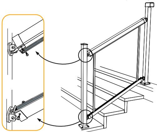
**3** Place a baluster into both rails near the bottom post - ensure that the baluster is plumb and 100 mm or less from the post. Starting from the bottom end of each rail, measure and cut the **end spacers** then remove the baluster (**Fig. 1**).
