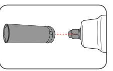
2 Push the socket onto the shaft until it clicks into place.
