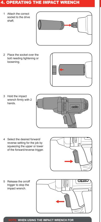
NOTE: WHEN USING THE IMPACT WRENCH FOR TIGHTENING, FIRST TIGHTEN THE BOLT OR NUT BY HAND TO PREVENT DAMAGING THE THREAD.
