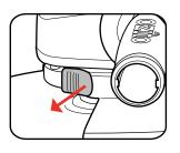
2. Align tabs on the guard with slots on the guard collar. Remove guard.
