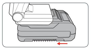
2 To remove, press and hold the battery release tab and pull the battery away from light.
