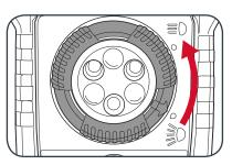
2 For a wide beam, rotate the beam setting dial clockwise " 글 ●".
