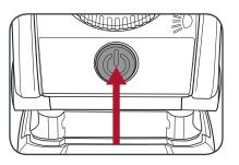
2 To turn the light off, press the on/off switch again.
