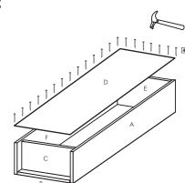
\*NOTE\* FOLD OPEN BACK AND PLACE ONTO UNIT MAKING SURE TO KEEP IT PARALLEL TO THE TOP AND SIDES OF THE UNIT. ATTACH USING THE NAILS
