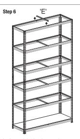
Apply remaining brackets as above to desired height. Ensure that braces 'E' are fixed to all shelves
