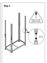
Place MDF board on bottom shelf to minimise buckling. Join the upper legs to the lower legs with the connector pins. Note: The legs are designed to sit directly on top of each other - don't overlap them. Handy Hint: Flathead screwdriver may be used to tap in connector pins.
