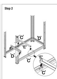
Use shelf bracket 'D' for the side brackets using the shelf bracket from Step 1 as a guide for height. Allow 1 keyhole free from the ground as shown in the diagram. Use same shelving brackets for opposing sides as shown in the diagram. Place brace 'E' as shown.
