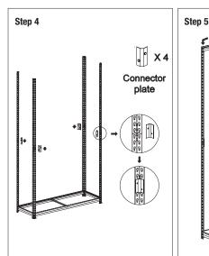
Join the top rivets of the connector plates to the bottom keyholes of the upper legs and bottom rivets of the connector plates to the top keyholes of the lower legs. Gently tap the connector plates in place with a mallet and a screw driver on the notch.
