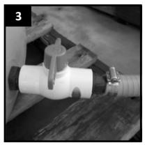
Screw one end of the Flexible Suction Hose onto the Ball Valve. (Check all hose clamps are fully tightened).
