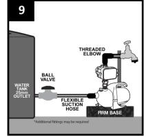
Screw the Brass Tap onto the end of pipe (not supplied) and secure to the ground with a metal or wooden stake for stability.
