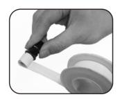
3. Screw the male nitto fitting clockwise into the female end of the air inlet.
