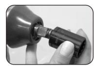
Note: The impact wrench should only be used with impact sockets. Standard sockets may shatter and break.
