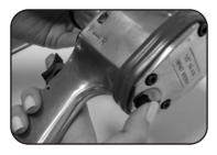
2. To turn the wrench on, squeeze the on/off trigger. To turn off, release the on/off trigger
