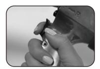
3. To restrict the air flow turn the regulator valve to a lower setting.
