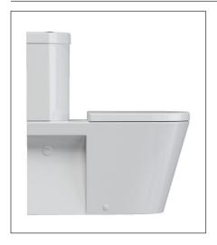
A softened geometric designed wall faced toilet suite conceals plumbing fittings for a clean and modern look. The pan connection system includes the patented Caroma Uni-Orbital® Connector for increased installation flexibility. The Caroma Uni-Orbital® Connector extends to any position in a 50mm radius, unlike traditional connectors that only move backwards and forwards. The setout range is from 60mm – 195mm with a recommended setout of 140mm.
