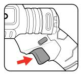
3. To stop the saw, release the on/off trigger
