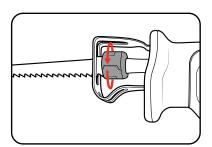
4. Pull on the blade to ensure it is properly secured.
