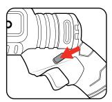
2. Squeeze the on/off Trigger
