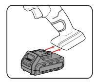
2. To remove, press and hold the battery release tab and then slide out
