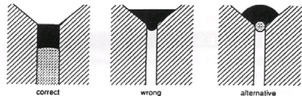
In corner joints too, the insertion of a release tape or backer rod is required, otherwise the sealant will fall during expansion of the joint.
