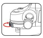
2 Align tabs on the guard with slots on the guard collar and then remove guard.
