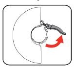
3 Tighten guard nut then close the guard lever.
