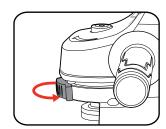
NOTE: IF THE GUARD NUT IS OVER-TIGHTENED, THE GUARD LEVER WILL NOT BE ABLE TO CLOSE PROPERLY.
