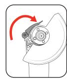
2 Tighten guard by pressing the lever down.
