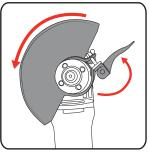
1 Loosen guard lever, align tabs and rotate guard to the required position.
