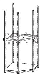
Fix brackets 'A' so that the top rivet sits on the upper legs and the bottom rivets sit on the lower legs. Repeat with brackets 'B' and 'E', followed by brace 'G' as done previously.
