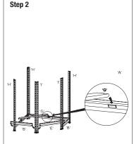
Use two shelf brackets 'B' for the side brackets using the shelf bracket from Step 1 as a guide for height, followed by shelf bracket 'E' as shown in the diagram. Place brace 'G' as shown.
