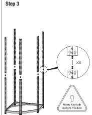
Join the upper and lower legs with the connector pins, as shown in the diagram, taking into account upright position. Note: The legs are designed to sit directly on top of each other – don't overlap them. Handy Hint: Flathead screwdriver may be used to tap in connector pins.
