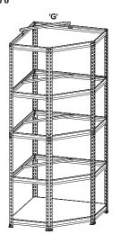
Apply remaining brackets as above to desired height. Ensure that brace 'G' are fixed to all shelves.
