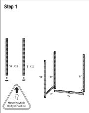
Place foot end caps onto the bottom of the 5 legs 'H' and 'l'. Note upright position. Place shelving bracket 'A' onto the legs. A rubber mallet can be used to lightly tap all brackets into the keyholes of the legs into place. Allow one keyhole free between the foot cap and the shelving bracket.
