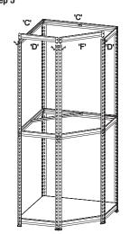
Fix brackets 'C', 'D' and 'F' at the very top allowing room for the MDF board to sit flush against the legs. Repeat as per previous step.
