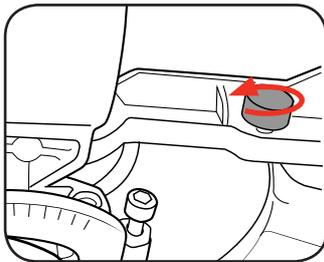
2. Rotate the mitre table to the desired angle using the mitre angle scale.
