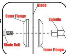
9. Fit the new blade onto the spindle taking care that the inner flange sits behind the blade.
