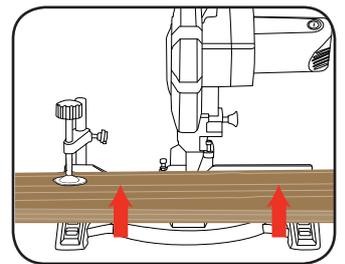
Material clamp will assist when making cuts when feeding materials from either side of the saw.
