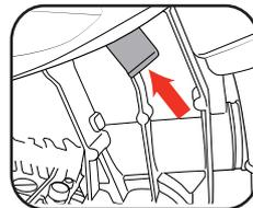
**Note:** The spindle lock button holds the blade in place when using the hex key to change the blade.
