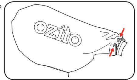
2. Slide the end of the dust bag over the dust extraction port and release the clamp.
