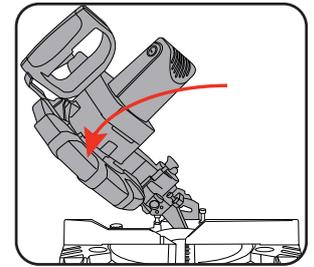
3. Tighten bevel lock knob at selected angle
