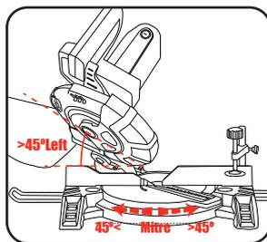
**Note:** To obtain good cuts when performing bevel or compound cuts the workpiece should be clamped.
