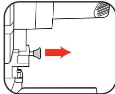
3. Using the 5mm hex key loosen and remove the screw that secures the blade bolt cover.
