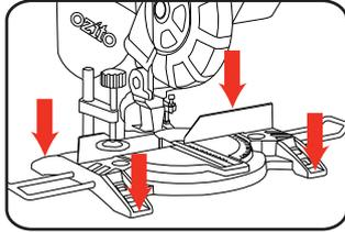
**Note:** If required, the Mitre Saw can be mounted onto a 13mm piece (or thicker) of plywood which can then be clamped to the work bench or mitre saw stand. This provides the flexibility to transport the Mitre Saw to other work areas.
