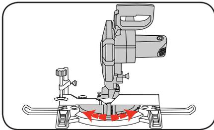
**Note:** The mitre table features positive click stops at 0°, 5°, 10°, 15°, 22.5°, 30°, 35°, 40° and 45° for quick setting of common mitre angles.
