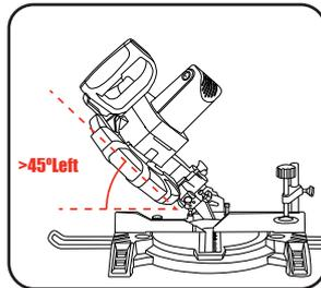
A compound mitre cut involves using a mitre angle and a bevel angle at the same time.
