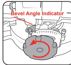
2. Tilt the cutting head to the desired bevel angle as shown by the bevel angle indicator.
