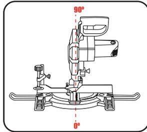
Mitre cuts are made with the mitre scale set at an angle other than 0° either to the right or left
