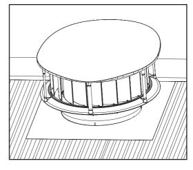
Ensure that the flashing covers the roof corrugations or ribs equally and that it is located between roof rafters.
