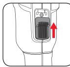
2 To use the lock on function, slide the lock-on switch to the full forward position.
