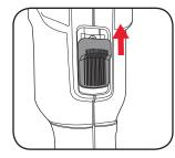
3 To turn off, Push the rear of the switch and the switch will automatically spring backwards into the off position.
