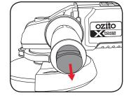
2 Depress and hold the spindle lock to prevent the spindle rotating.
