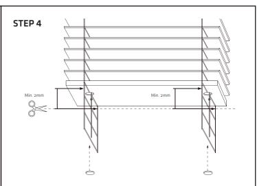
Cut excess ladder and cords. Cut ladder at least 2mm under the last cross ladder. Re-install bottom rail plugs.
