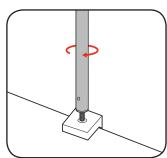
4 Ensure that the tool stand is secure and then hang the rotary tool onto the hook by the hanging ring.
