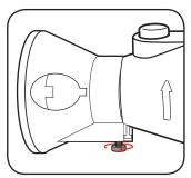
5 Adjust the drilling depth to the desired height.
