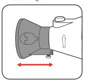
Secure the depth by tightening the depth locking screw.
