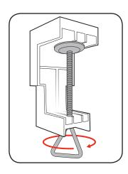
2 Place the desk clamp onto the desk and tighten the clamp.
