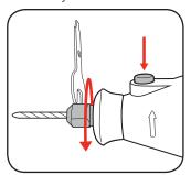
3 Screw the cutting guide onto the rotary tool.
