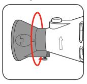
4 Loosen the depth locking screw.
