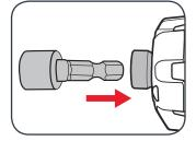
3 Release the drive bit retaining ring then pull on the bit to ensure it is firmly in place.
