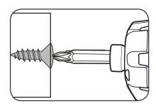
**Note:** Do not force the driver or apply side pressure to elongate the hole. Let the impact driver do the work.
