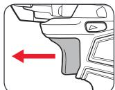
3 Control the speed by adjusting the amount of pressure applied to the trigger.
