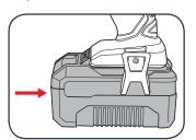
2 To remove, press and hold the battery release tab and then slide out.
