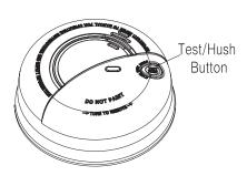
DO NOT stand close to the Alarm when the horn is sounding. Exposure at close range may be harmful to your hearing. When testing, step away when horn starts sounding. Push and hold the Test/Silence button on the cover until the LED flashes. The alarm horn will sound 4 beeps, a pause, then 4 beeps. The ALARM (RED) light will flash.
