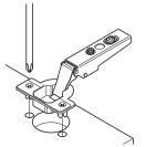
Cup fixed with pre-mounted spreading dowels.
