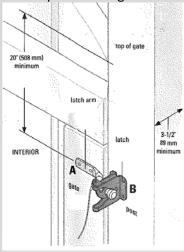
**B** Secure latch assembly with supplied screws.
