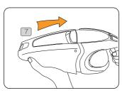
Allign bottom of the dirt container first and clip nozzle on.
