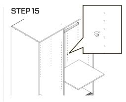
Insert plastic shelf supports into pre-drilled holes at the desired shelf heights then slide shelves into place
