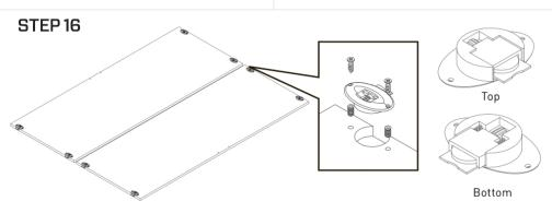
Insert lugs into the screw holes at the top and bottom of the door panels.
