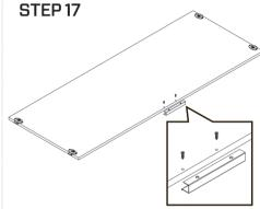
Attach door handles to doors holes using 16mm screws
