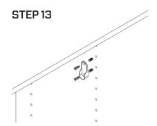
Attach aluminium hanging rail brackets by pushing plastic lugs into holes at the desired height. Screw the brackets into the lugs using 16mm screws
