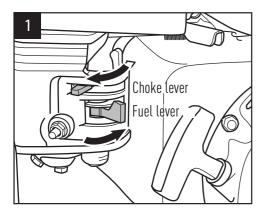
Move the choke lever to the left/closed position and fuel lever to the right/open position..
