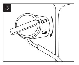
Turn the engine on/off switch to "ON" position
