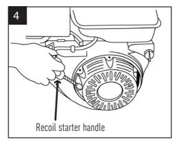
Start the engine as follow: Hold the recoil starter handle firmly and pull it slightly until the compression position is reached,
