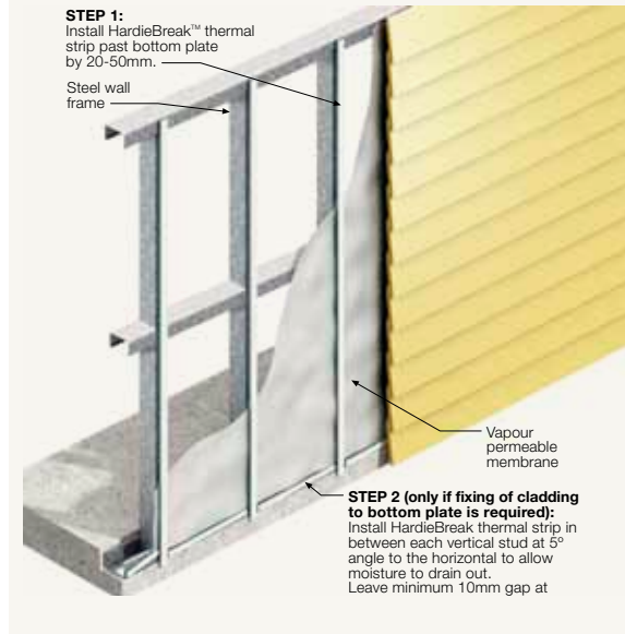
Figure 26 Installation of HardieBreak™ Thermal Strip for weatherboards and planks direct fixed
