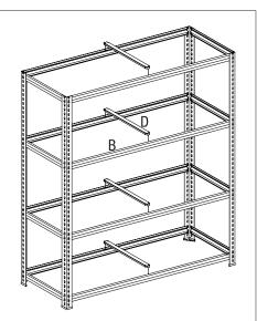
Step 4: Slot Braces (Part D) into position through the holes provided on the Long Beams (Part B).
