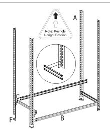
Step 1: Assembling bottom of frame
