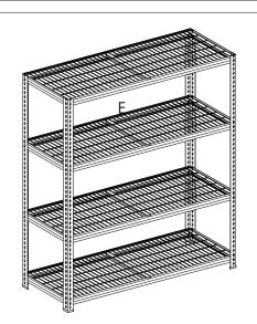
Step 5: Lay the Wire Shelving (Part E) between the Beams as shown.
