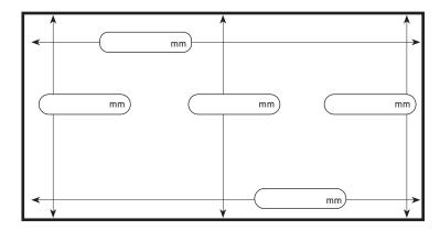
**Note:** Provide measurements of internal door frame as indicated on diagram.
